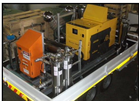
Mobile 18m 3 /h Oily Water Separator solution
